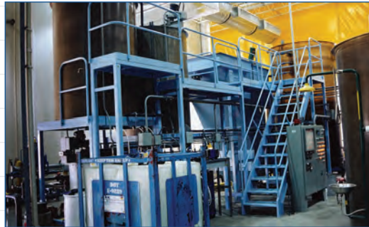
Continuous sedimentation wastewater treatment systems, offered in slant-plate (left) or tank-style designs (5-500 gal. per minute).
